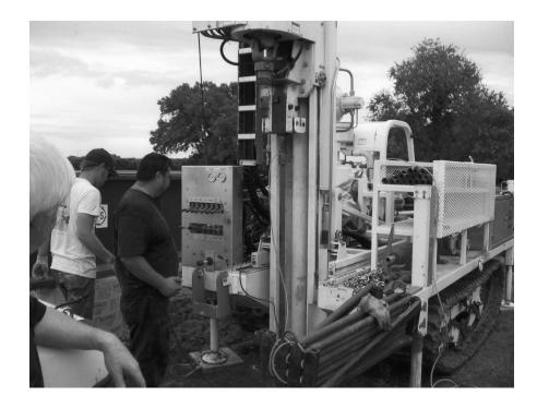
Figure 3.22- CPT Rig Performing Test on Site
