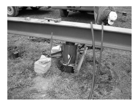
Figure 4.15 - Field Testing of the Pressed Steel Piles
