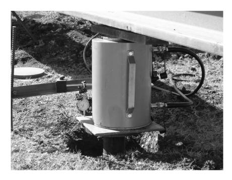
**Figure 4.10 - Field Testing of Helical Anchors**
