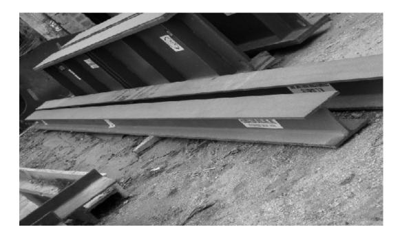
Figure 3.27- Reaction Beams for Underpinning Testing
