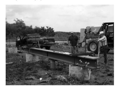
Figure 4.4 – Load Testing of Belled Shafts
