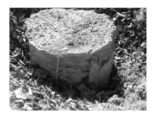
Figure 5.1 – Pushing Steel Rod Adjacent to Drilled Shaft
