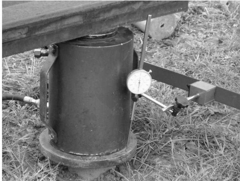
**Figure 4.18 - Field Testing of the Pressed Concrete Piles**
