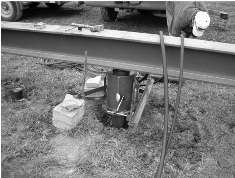
**Figure 4.15 - Field Testing of the Pressed Steel Piles**
