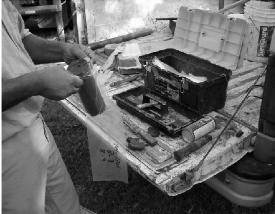
**Figure 3.9- Recording of Shelby Tube Samples**
