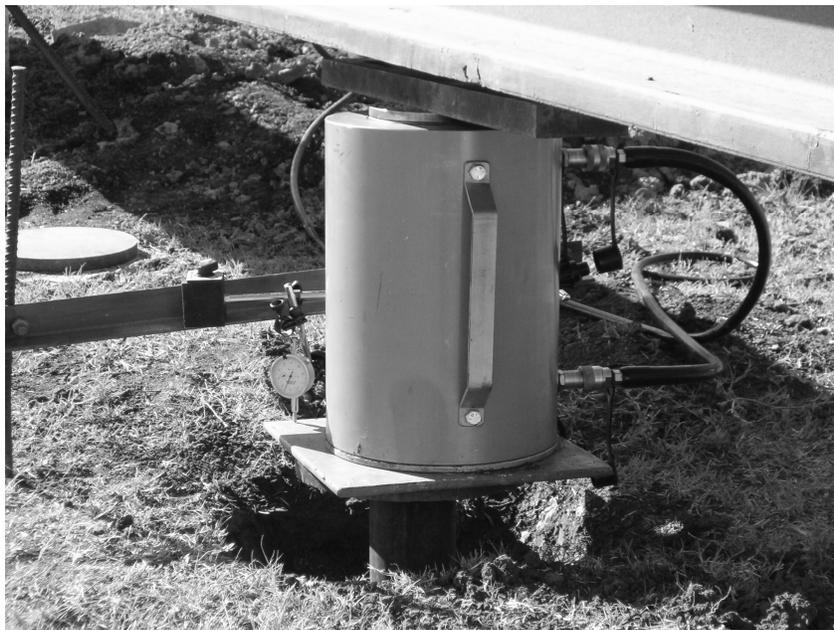
**Figure 4.10 - Field Testing of Helical Anchors**
